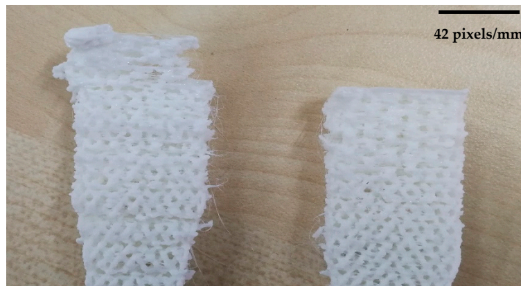
Figure 11. Defect in 75° flat samples.
