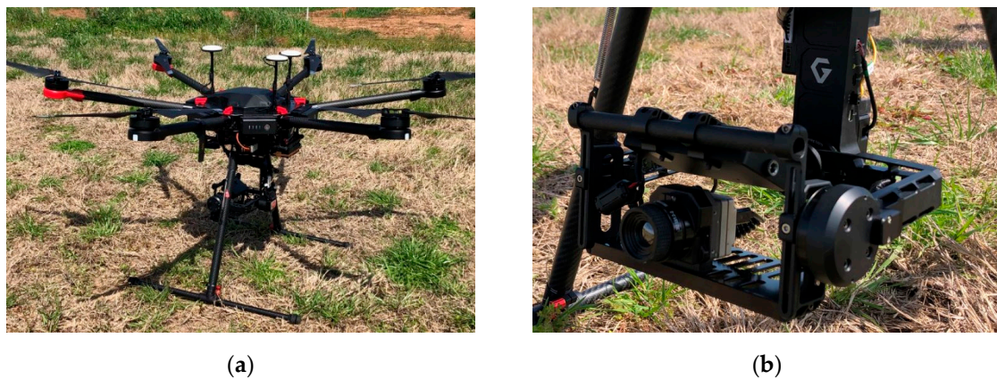
Figure 1. Unmanned aerial vehicle, (a) DJI Matrice 600 Pro and (b) ICI thermal camera.
