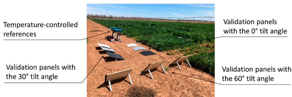
Figure 6. Temperature-controlled references, three sets of three-colored square validation panels placed on the ground at different tilt angles, and ground-truth temperature measurements.
