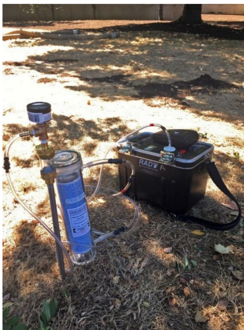
Figure 1. RAD7 soil gas testing setup.
