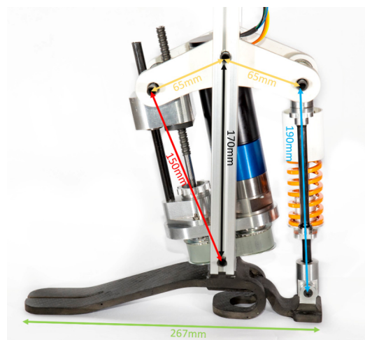
Figure 5. An image of the prototype of the ankle-foot prosthesis with the main dimensions (the actuator and shock-absorber dimensions refer to the condition at \gamma = 90^\circ ).
