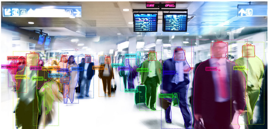
Fig. 1 Use of computer vision technologies to capture individuals on their way to the departure gate by localising their facial features and comparing them to existing data base entries
