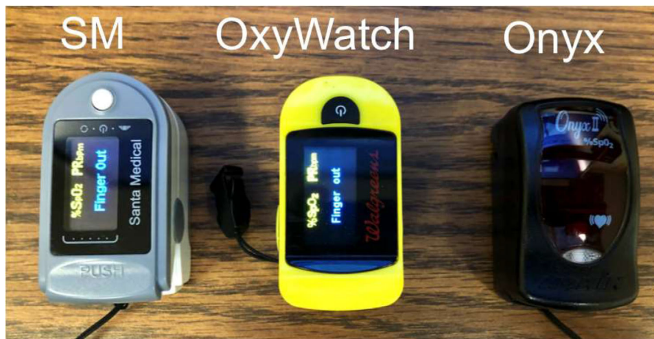
FIGURE 1 The 3 portable pulse oximeters used in this study. From left to right: Santa Medical SM-165 (SM), Walgreens' OxyWatch C20 (OxyWatch), and Nonin Onyx II 9550 (Onyx)
