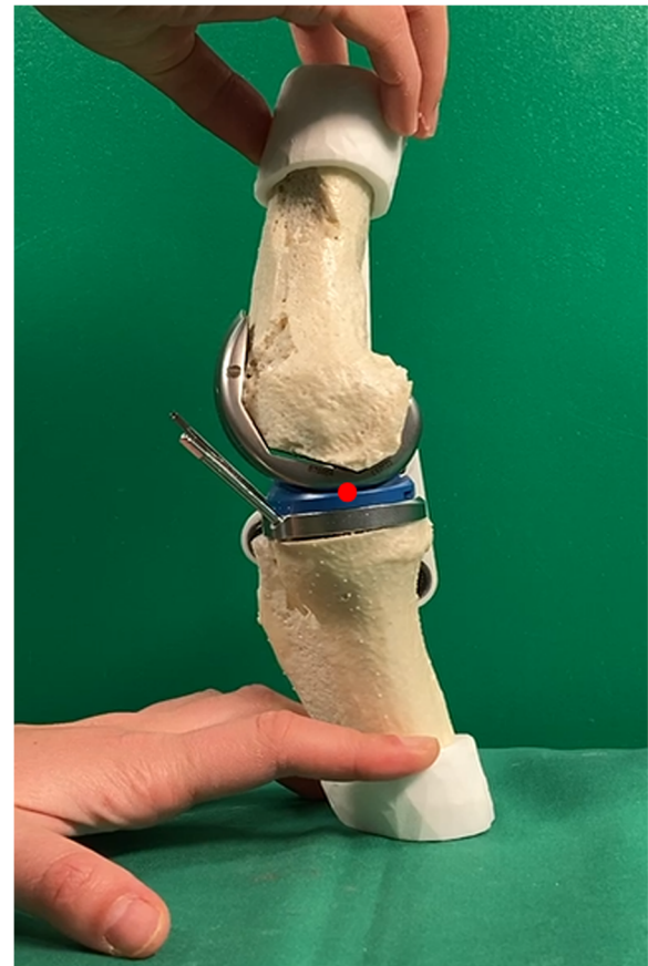
Fig. 10 Knee model after surgery, shown in the sagittal plane with the measured contact point (in red) between femur and tibia
