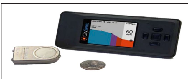
Figure 2. The Eclipse ICGM System was developed by Glysens, Inc. The implantable continuous glucose monitoring system (left) accurately measures the concentration of tissue fluid glucose, remains stable between infrequent recalibration periods, and reliably communicates with an external transmitter-receiver (right) using low-energy Bluetooth for more than one year ( www.glysens.com ).
