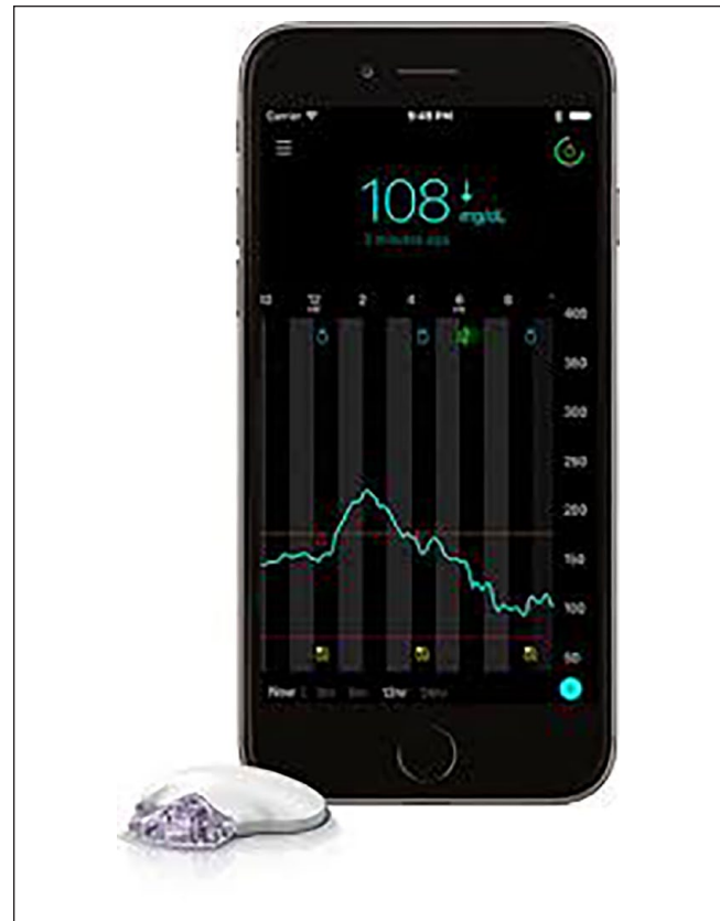
Figure 1. The Guardian™ Connect continuous glucose monitoring system displays sensor glucose data on a smartphone in real time and provides predictive threshold alerts 10-60 minutes before a preset low or high sensor glucose level, as well as threshold alerts when glucose reaches a preset low or high sensor glucose level. Sensor glucose data are recorded 24 hours/day and can be uploaded into CareLink™ Personal software for later review and analyses.
