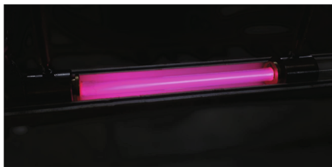
Fig. 2. Intense UV emission in the plasma discharge chamber.
