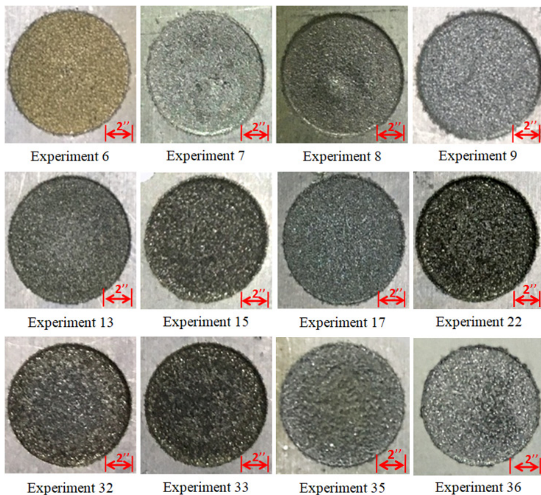
Figure 5. Machined surface of selected experimental trials.
