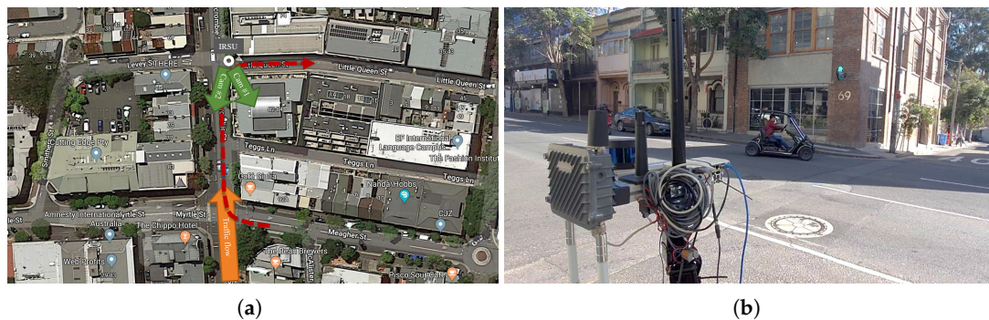
Figure 13. Experiment setup at the intersection of Abercrombie St and Little Queen St. In (a), the IRSU was setup facing south of Abercrombie St. The car traffic flow was going north on this one-way street. The trajectory of the CV is denoted by a dashed red line, which indicates that the CV turned from Meagher St to Abercrombie St, followed by Little Queen St. In (b), CPMs were transmitted from the IRSU to the moving CV through Cohda Wireless MK5 devices.
