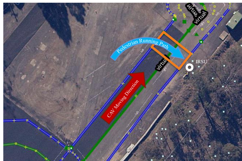
Figure 20. Experiment setup in a lab environment. It is shown in the Lanelet2 map and lidar feature map built for the experiment site, which contains the road boundaries and lanes information. The light blue dots distributed in the bottom right corner represent the locations of observed features in the environment (trees, poles, corners of structures). The designated pedestrian crossing area is labelled as an orange rectangle.
