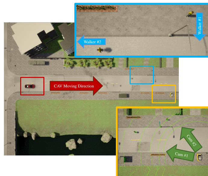
Figure 16. Experiment setup in the CARLA simulator. The CAV, a red car, moved to the east direction towards two walking pedestrians and an IRSU deployed on the roadside. The IRSU was spawned in CARLA as a mini car parked on the roadside.
