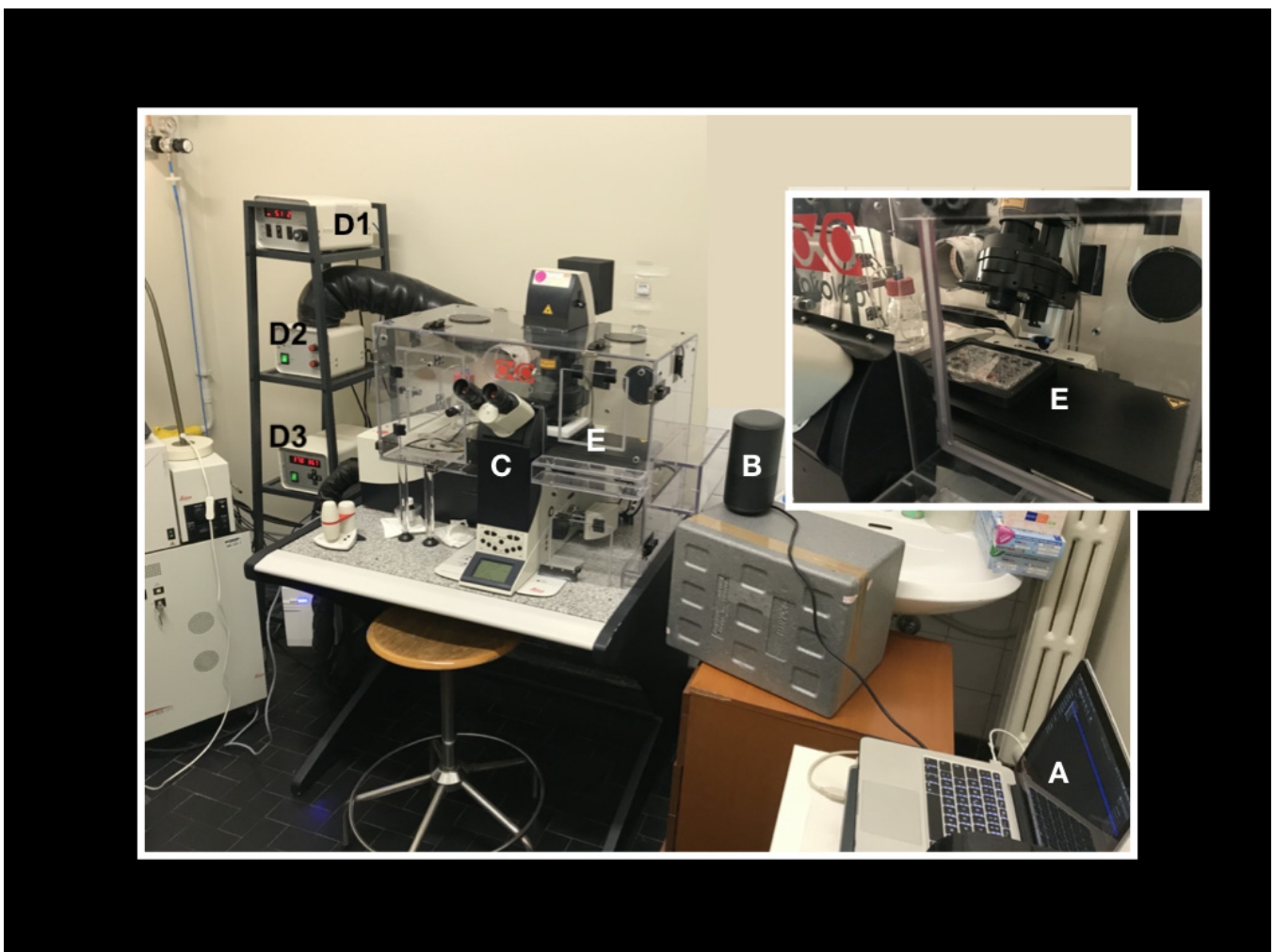
Figure 5. Our laboratory set up for the experiment. A laptop computer with the audio tracks (A) is connected to an amplifier (B) positioned nearby the microscope (C) and its incubator (E). With a phonimeter we calibrated the volume of the amplifier so that the intensity of the sound in the point where the cells are positioned (E) is about 60 dB, which corresponds to a normal vocal conversation. (D1) CO 2 controller, (D2) heating unit, temperature control unit (D3). We remark that also “control cells” were exposed to the speaker plugged to energy without any sound produced in order to exclude that our findings could be the result of any small vibration produced by the speaker itself instead of the sound. Finally, the vocal sounds used were pronounced by 3 different people, giving the same results.
