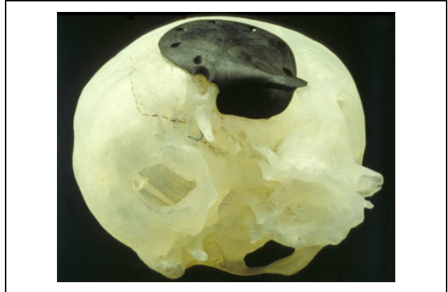
Figure 2. A CFRP implant (Medtronic-Sofamor Danek) on a stereolithographic defect model. The defect model was used to predetermine the position, direction, and length of the fixation screws. CFRP indicates carbon fiber-reinforced plastic.
