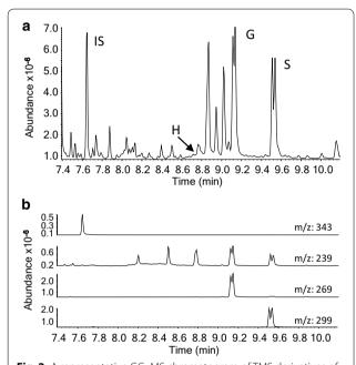
**Fig. 2** A representative GC–MS chromatogram of TMS derivatives of bagasse thioacidolysis products prepared by the modified method. **a** A total ion chromatogram. The double peaks of G and S represent the *erythro* and *threo* isomers of guaiacyl and syringyl units released by thioacidolysis. **b** Selected ion chromatograms for *m/z* 343 (IS), 239 (H monomer), 269 (G monomer), and 299 (S monomer). IS: Internal standard; H: *p*-hydroxyphenyl monomer; G: Guaiacyl monomer; S: Syringyl monomer
