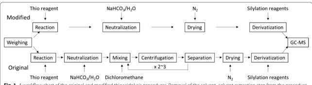
Fig. 1 A workflow chart of the original and modified thioacidolysis procedures. Removal of the solvent-solvent extraction step from the procedure reduces the time of sample processing and eliminates the use of the hazardous chemical dichloromethane
