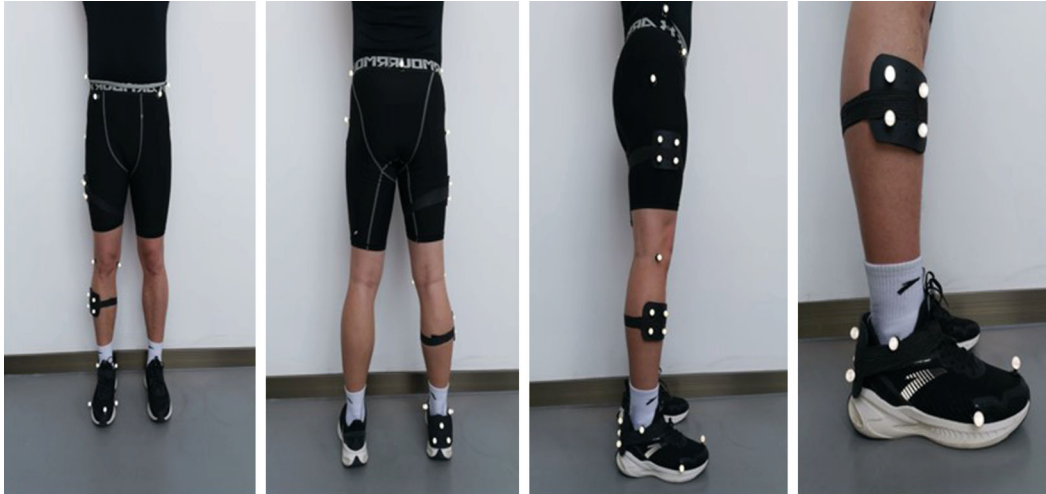
FIGURE 1: Placement of combined marker set consisting of retroreflective cluster markers and single 14 mm retroreflective markers.
