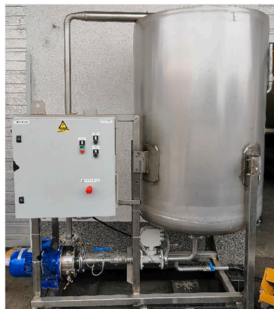
Fig. 3. Key elements of the test rig: 1 – RGHC, 2 – phase asynchronous motor, controlled by variable frequency drive, 3 – pressure side throttling valve, 4 – 1000 L tank, 5 – suction side throttling valve, 6 – discharge valve. Installed measurement equipment: a – absolute pressure transducer, b – differential pressure transducer, c – electromagnetic flow meter, d – hydrophone, e – high-speed camera.
