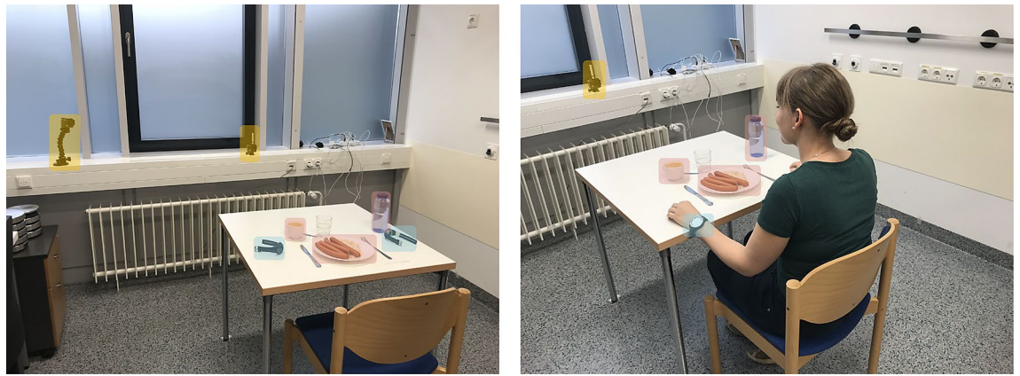
Figure 4. Figures depicting the EaC experiment setup. The picture on the left-hand side highlights the position of the two cameras (yellow). On the right picture, the researcher showcases the position of the smartwatch on the wrist (blue). In both pictures, the contents of the standardized meal are marked (red).
