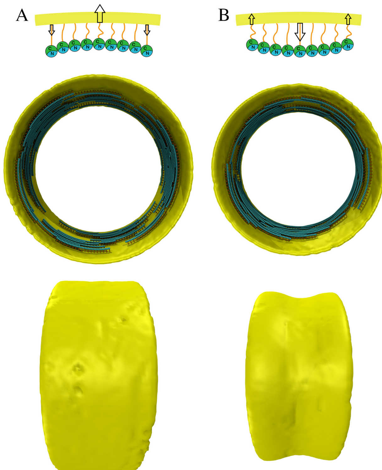
FIG 4 (A and B) Traditional bending (A) versus reverse bending (B). (Top) Schematic of how filament bending has traditionally been thought to occur versus bending in the opposite direction to the membrane (“reverse” bending). In both cases, the C termini face the membrane. Arrows indicate the directions of forces exerted on the membrane by the filament. (Middle) Simulation results after 100 s of systems in which the membrane initially had a diameter of 500 nm and the preferred curvature of the filament was 1/250 \text{ nm}^{-1} (twice that of the initial membrane). Traditional bending did not result in constriction, but reverse bending did. (Bottom) Side views.
