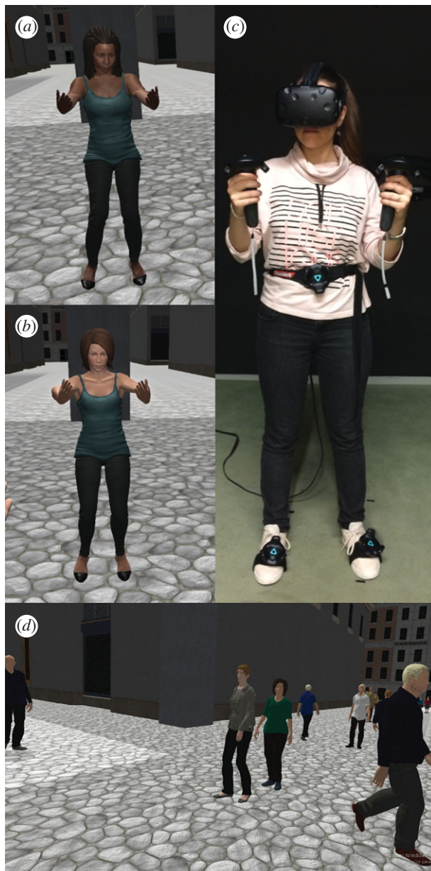
Figure 1. The scenario. (a) The participant embodied in a Black virtual body is in front of a mirror and carrying out embodiment exercises. (b) A participant in a White virtual body. (c) Showing the participant with the virtual reality equipment. (d) First-person view of the Negative crowd—note how two virtual women in the centre of the picture stare at the participant.
