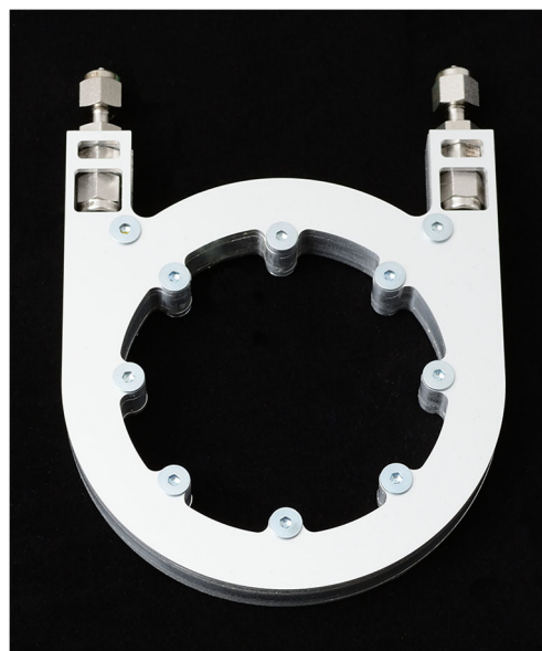
Fig. 3 Photo of the small aluminum GC "oven" (80 mm \times 105 mm \times 11 mm (width \times length \times height)) with 1/16" stainless steel bulkhead unions (top) for easy connection
