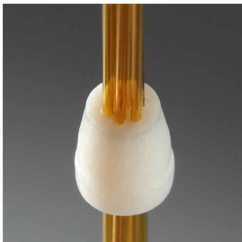
Fig. 2 Photo of the modified 1/16" PTFE ferrule with seven 0.5-mm bores and 250- \mu\text{m} -ID standard fused silica GC columns inserted (Rtx-Volatiles, Restek GmbH, Germany)
