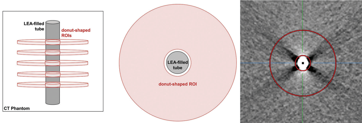
FIG 1. Schematic illustration of the donut-shaped ROI created by the MITK with an inner radius of 6 mm and an outer radius of 26 mm. The tube filled with the LEA of interest was placed centrally with a radius equal to the radius of the donut hole. For each tube, the measurement was performed with an ROI in 5 different positions according to the length of the LEA cast.
