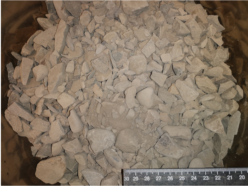
Fig. 11. Loose material tested with RLTTs.
