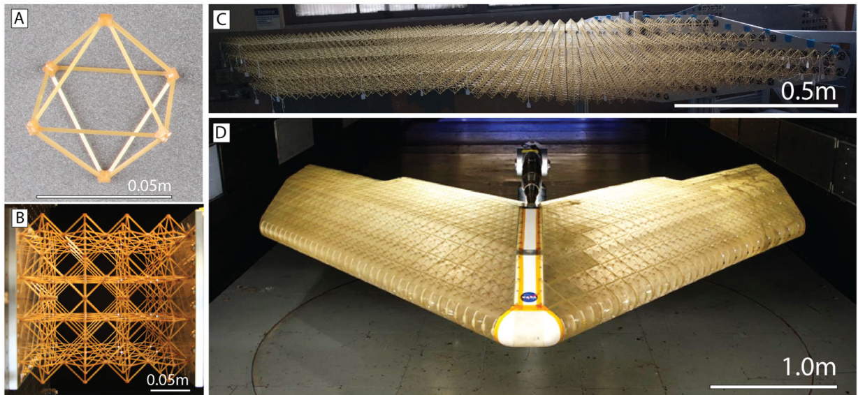
Figure 1: A large-scale, ultralight adaptive structural system. A) Modular building block unit, B) 4×4×4 unit cube during mechanical testing, C) Single half-span wing structure composed of 2088 building block units, D) Blended wing body aerostructure with skin, mounted to central load balance in the 14×22 subsonic wind tunnel at NASA Langley Research Center
