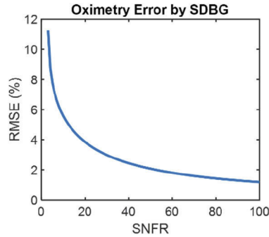
Fig. 6. RMSE of simulated sO 2 measurements with respect to the ground truth as a function of SNFR.
