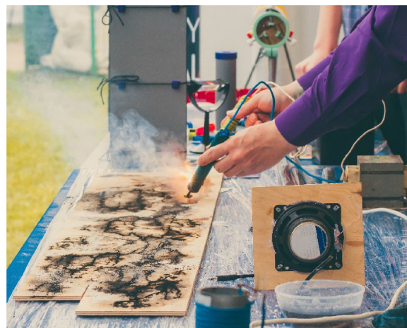
FIGURE 1 The process of fractal wood burning using a microwave oven transformer 4
