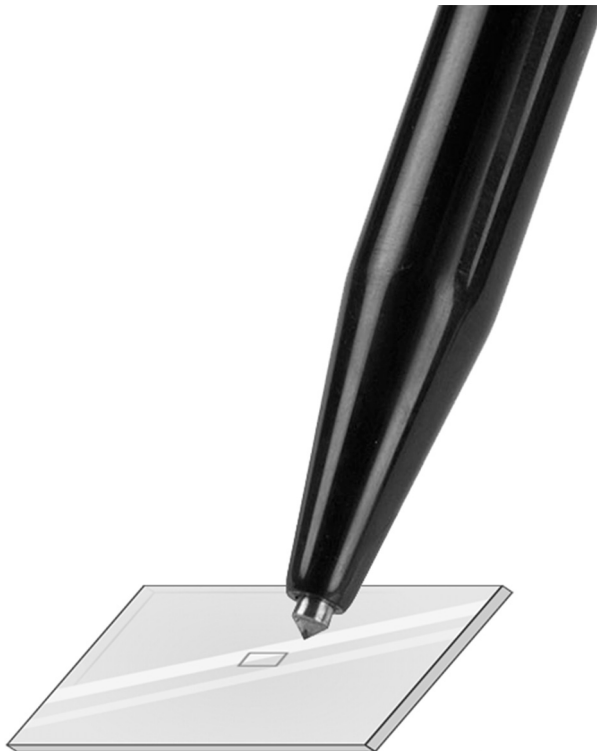
Figure 1. Schematic representation of how the square is drawn on the coverslip A glass-writing diamond pen is used, as indicated.
