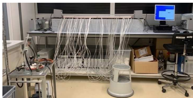
Figure 6. Biodegradability equipment (RespiCond™) at the Institute for Biodiversity and Ecosystem Dynamics (IBED) of the University of Amsterdam. The setup consists of 96 parallel respirometers in a temperature-controlled water bath under dark conditions. Photo by L. Filicetto.
