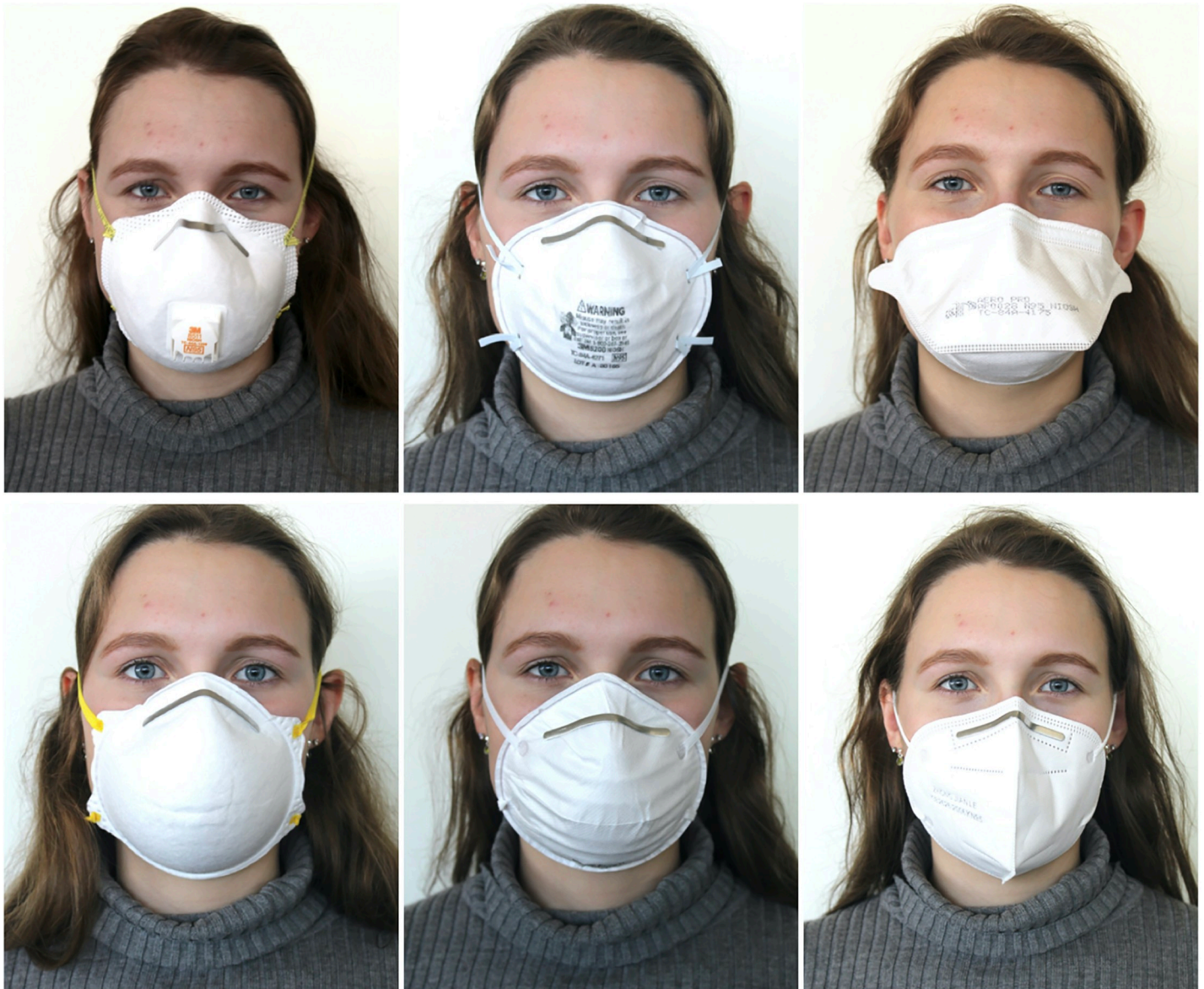
Fig 2. N95 and KN95 respirators tested. Top row, from left to right: 3M 8511, 3M 8200, Aero Pro AP0028. Bottom row, from left to right: Makrite 9500, Xiantao Zong ZYB-11, Zhong Jian Le KN95.
