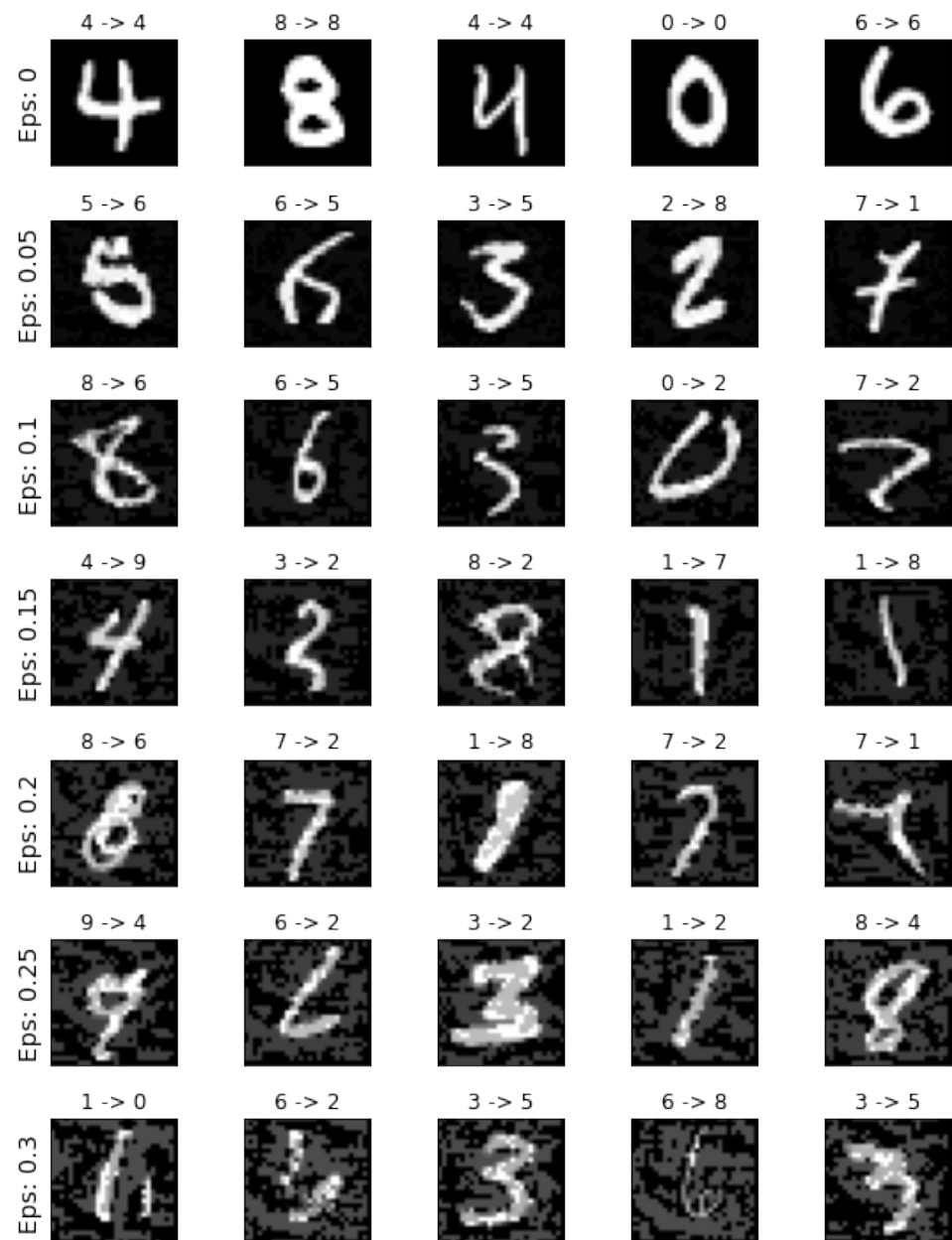
Figure 8. Fast Gradient Sign Attack (FGSM) on the MNIST dataset. The first row contains unperturbed images, while in the subsequent rows are perturbed using some \epsilon value, resulting in the model misclassifying them.
