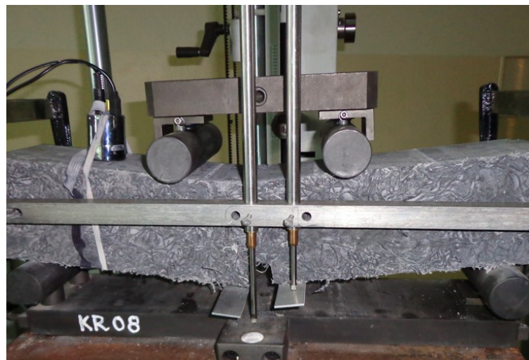
Figure 9. The four-point bending test, paste ZV_f6\% after the test.
