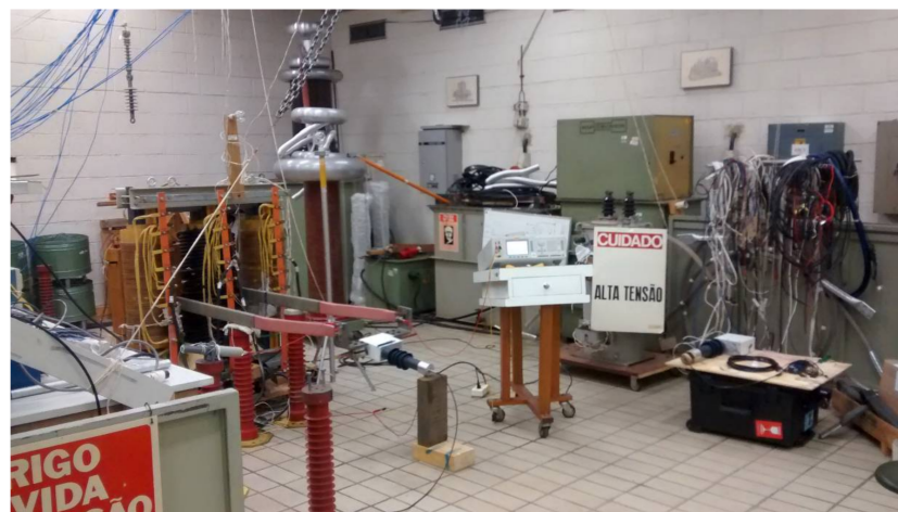
Figure 6. Set-up used to characterize the sensor in a high-voltage laboratory.
