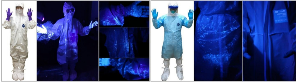
Figure 2. Consecutive scenes of contamination in the doffing process comparing adapted practice and enhanced protocols. Note: First picture (from left), Level D kit donning completion with accustomed practice; Second picture, checking contamination in the darkened room with UV lights immediately after finishing a minimum 1-minute patient care simulation; Third picture(s), while checking contamination result, severe contamination found on the left glove and the left sleeve of coverall (top), on the front area of coveralls (middle; in particular on the coveralls placket), and on the right glove and the right sleeve of coveralls (bottom); Fourth picture, Level D kit donning completion with enhanced protocols (eg, disposable long-sleeve apron); Fifth picture, severe contamination found on the disposable long-sleeve apron's front surface; Last picture, clean coveralls surface after doffing a disposable apron and outer gloves.
