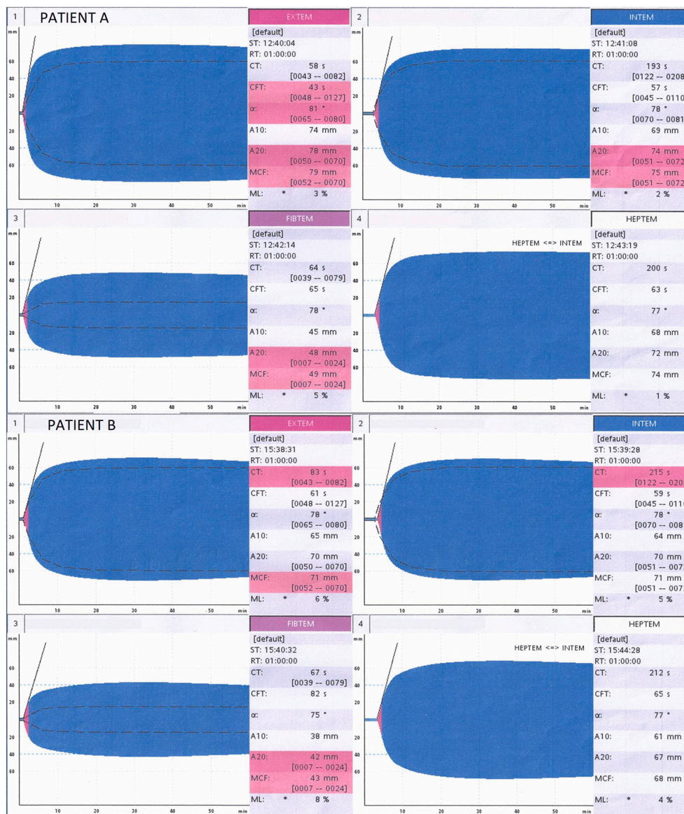
Fig. 1. ROTEM for patients A and B. EXTEM, extrinsic pathway; INTEM, intrinsic pathway; FIBTEM, fibrinogen activity with platelet inhibitor; HEPTTEM, heparin inhibition with heparinase.
