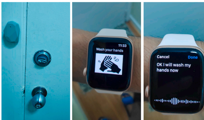
Fig. 7. iWash implementation, with the beacon fitted at the door, user receiving reminder on the smartwatch and responding via voice interaction.
