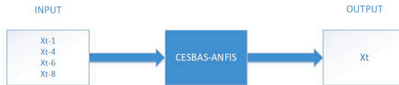
Fig. 10. Input and output visualization of proposed CESBAS-ANFIS method.
