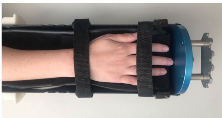
Fig. 1 Photograph of the hand cast used in Bone Metabolism Laboratory, Rheumatology Department, Faculdade de Medicina, University of São Paulo. A palm down orientation is used to evaluate 2nd and 3rd MCP (metacarpophalangeal) and PIP (Proximal Interphalangeal) joints
