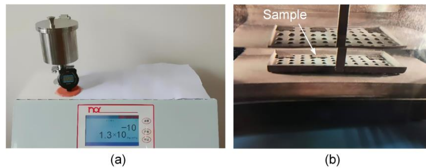
Figure 9. Leakage detection of SiC cavity structure: (a) the fine leak detection; (b) the coarse leak detection.
