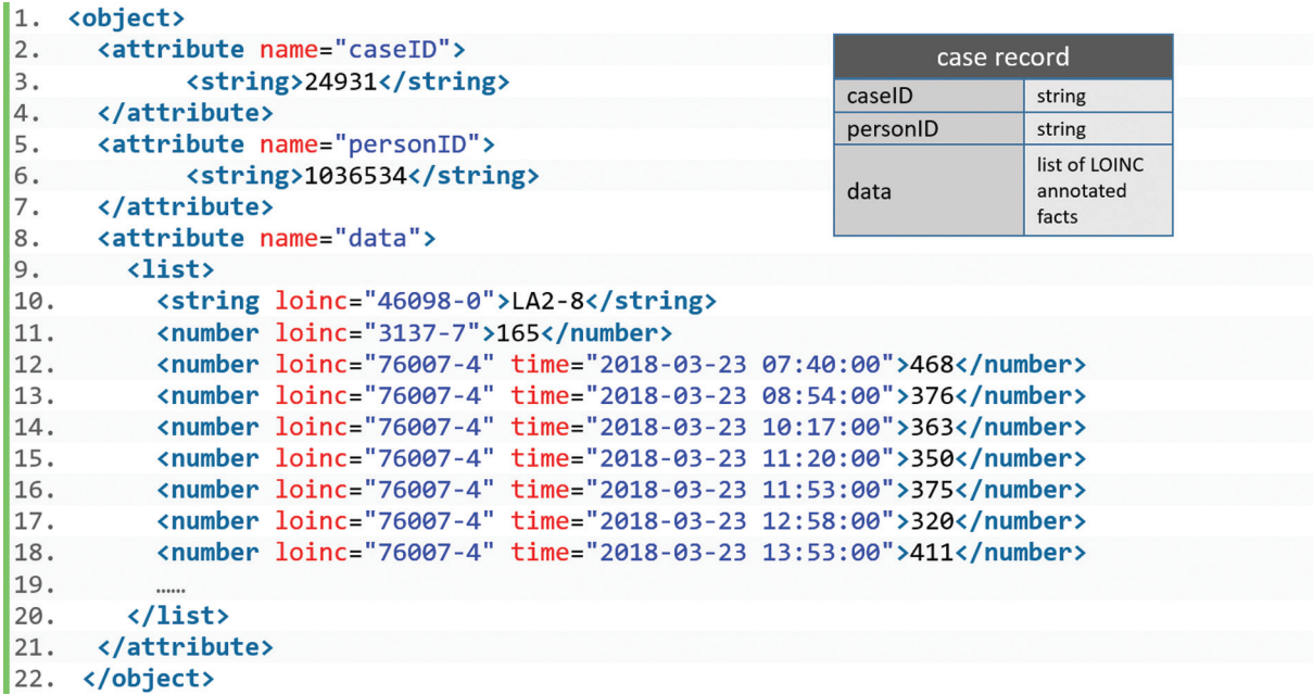
Fig. 1 Basic structure of a case record and its PLAIN Data Markup Language (PDML) representation.
