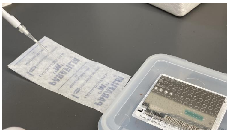
Figure 7. Preparation of samples for MALDI-TOF. Mix peptides with matrix on parafilm and transfer to MALDI plate.
