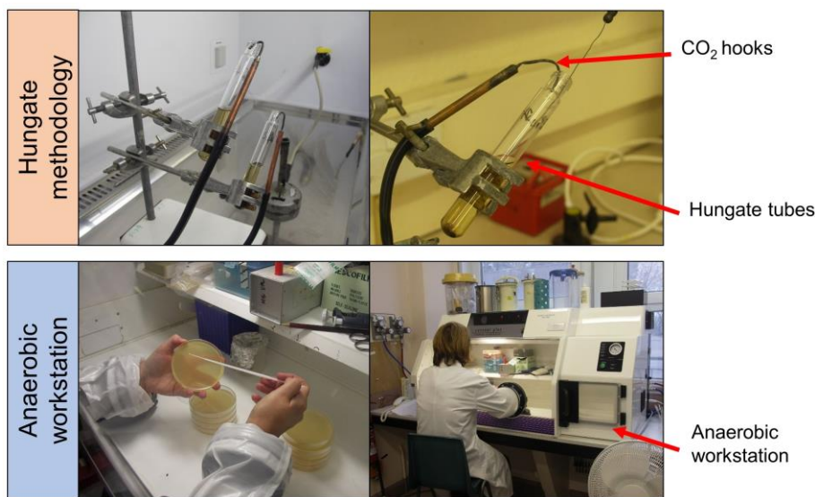
Figure 1. Culturing of strictly anaerobic bacteria using the Hungate methodology (growth in tubes) and anaerobic workstation (growth on Petri plates)
