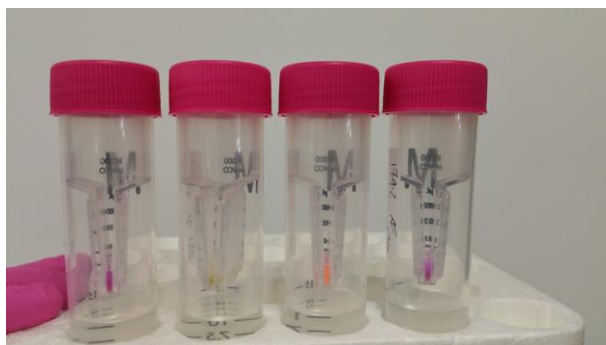
Figure 20. Concentrated FAST proteins. Image of FAST proteins in centrifugal concentration tubes. Highly concentrated FAST proteins can be seen even using visible light. From left to right are mCherry, mCitrine, mOrange, and mCherry.
