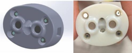
Figure 3: Design of the probe in SolidWorks and the prototype
