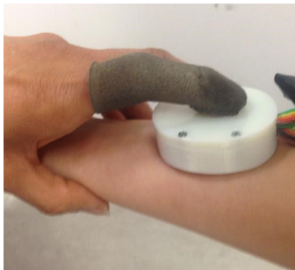
Figure 4: Use of probe and the pressure sensors over human tissue
