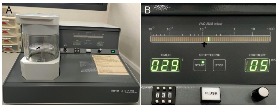
Figure 4. Glow Discharge. A. Glow Discharge unit BALTEC CTA 005. The black arrow indicates the position of the grid inside the chamber. B. Glow Discharge settings.
