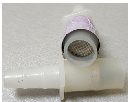
Figure 4. The “female” part of the pair of Nalgene Quick Disconnect, fitted on its wide end with monofilament cloth Nylon Mesh (1 mm opening). The silicon tubing is used to attach it to the Falcon tubes used as arms.
