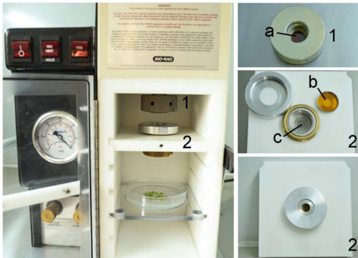
Figure 2. Side view of PDS-1000/He™ Biolistic Particle Delivery System. Before performing particle bombardment, the Petri dish containing Arabidopsis leaves was moved into the PDS-1000/He™ Biolistic Particle Delivery System (left). Part 1 and part 2 of the system were zoomed in at right. a is 1,100 psi rupture disk. b is microparticles carrier disk, which carries 1.0 \mu\text{m} Gold Microcarriers. c is stopping screen.
