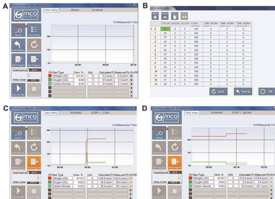
Figure 5. Programming gas compositions using the MCQ Gas Mixture Creator PRO software. A. Opening page of MCQ Gas Mixture Creator PRO software. B. The job program editing page (after selecting 'Edit Program'). To model intermittent hypoxia, N 2 (CH1) was set to 87% or 95% per line, O 2 (CH2) was set to 8% or 0% per line, and CO 2 (CH3) was set to 5%. Flow rate was set to 500 SCCM (equivalent to ml/min). Time work was set to 5 min per line. C. The running program after selecting 'Run Program', starting with 87% N 2 , 8% O 2 , and 5% CO 2 . D. The running program when oxygen conditions alternate to 95% N 2 , 0% O 2 , and 5% CO 2 .
