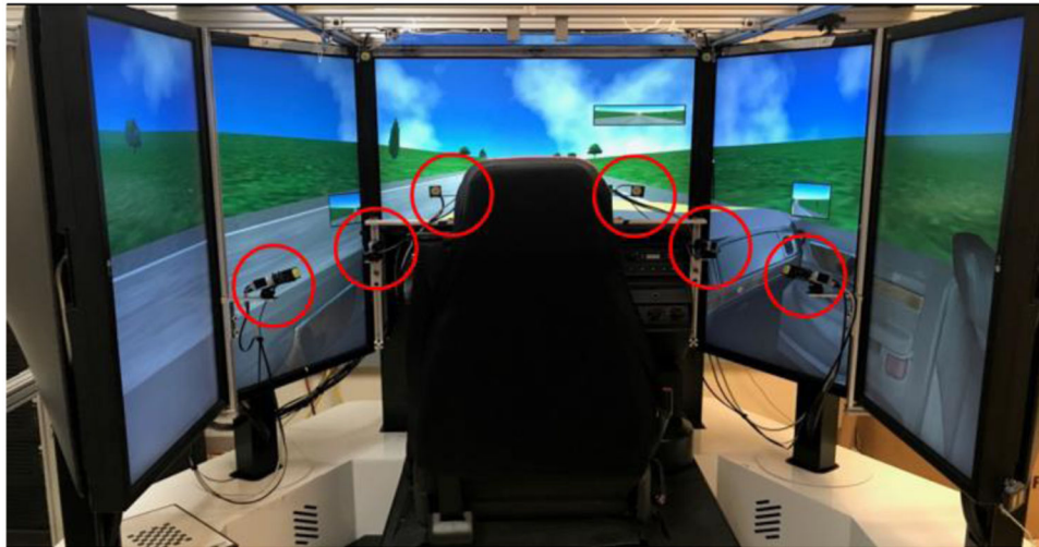
Figure 2. Image of the driving simulator equipped with 6 cameras (red circles) located around the driver's seat (two on the left, two on the right, and two in the center), which enabled recording of lateral eye and head position up to 90° to the left and right of the driver.
