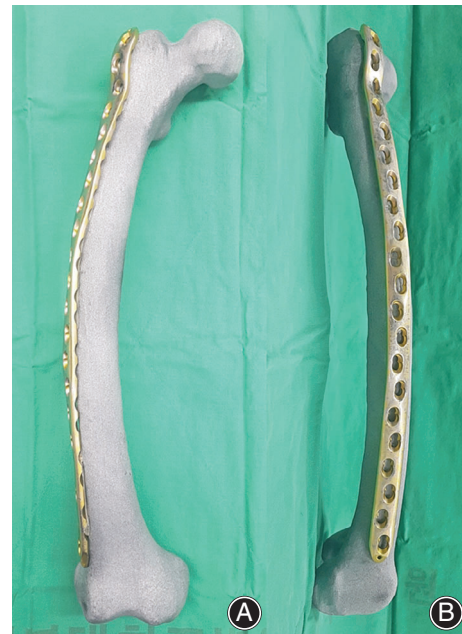
Fig. 3 Precontoured plate for patient 1. The locking compression plate was precontoured according to the shape of the bone model. Because of the three-dimensional complex deformity of the severely bowed femur, the proximal part of the precontoured plate was placed on the anterolateral aspect of the proximal femur. (A) Anteroposterior view. (B) Lateral view.
