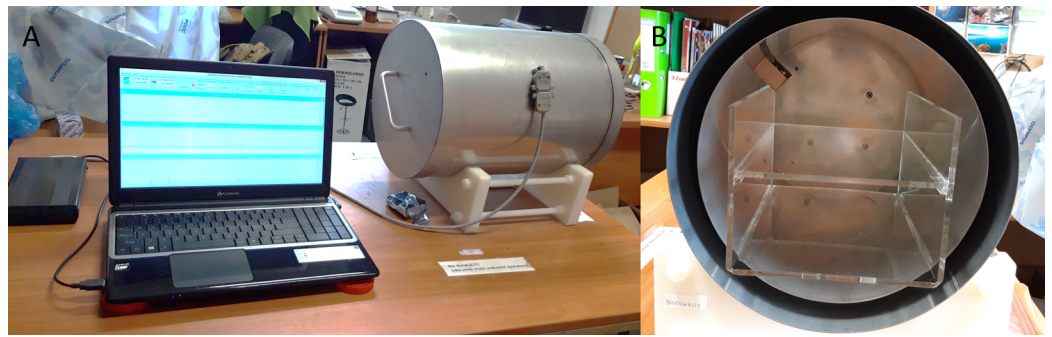
Figure 1 Chamber Isolated from the Magnetic Field (CIMF). (A) CIMF chamber during work, connected with a laptop, (B) inside view of the CIMF chamber, with shelves for test objects. The internal size of CIMF is 26.2 cm in diameter and 35 cm in length. Full-size DOI: 10.7717/peerj.10630/fig-1
